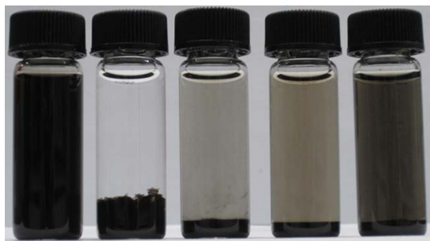
Figure 5. Photographs of aqueous suspensions of reduced GO, from left to right, reduced by L-AA, D-fructose, sucrose, glucose, and Na 2 SO 3 after storage for 1 month.
